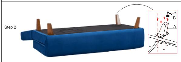
Insert all four screws before fully tightening.
