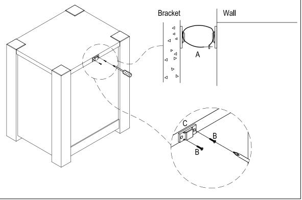
FINAL Step: Attach anti tilt strap or bracket to wall
