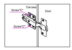
How to fix it - To move the door towards or away from the horizontal panels, loosen Screws "C". Adjust the door and then tighten Screws "C".
