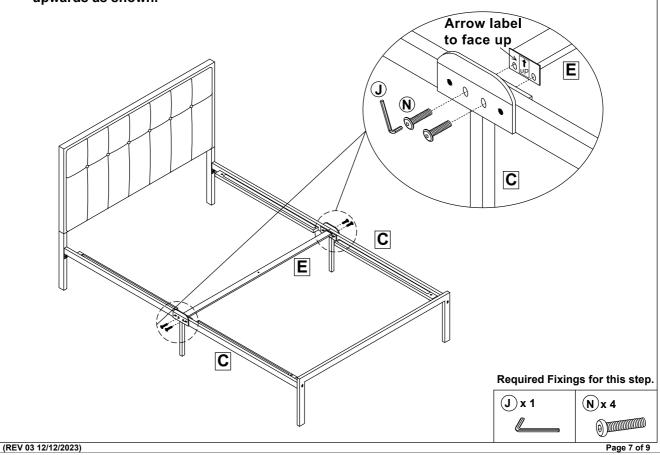
• Position central support system and secure as shown.
