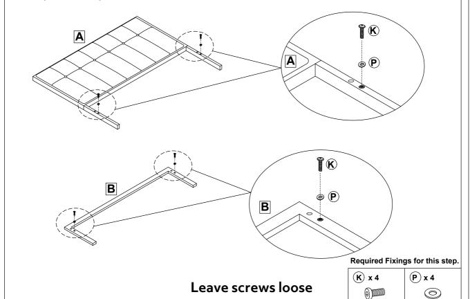
• Unfold and extend the side rails.
